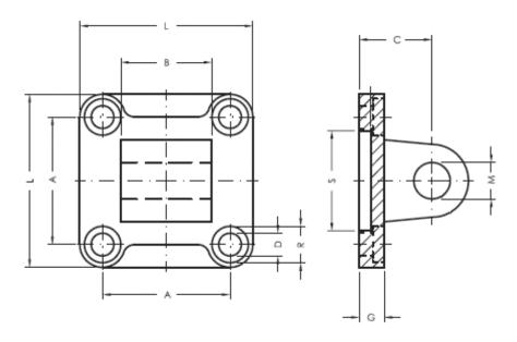
= 72.0 R = 18 Α В = 50 Countersunk screw = 36 Cylinder size = 80 = 11.0 D = 14 G L = 95 Μ = 16
